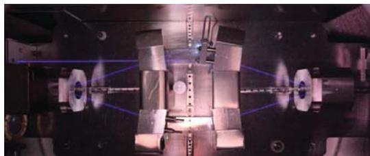
**Figure 1.** Picture of Mini-Ring. The light emitted along the Ar<sup>+</sup> beam trajectory is due to collisions with nitrogen gas injected into the vacuum chamber at pressure of about 10<sup>-4</sup> mbar. The blue light is due to the excitation of the N<sub>2</sub> molecules. The MCP imaging detector is placed at bottom left. A small spot due to neutralized Ar is well observed on the MCP.
