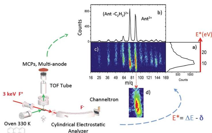
Fig.1 Experimental setup and the spectra:
