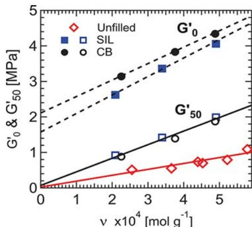
**Figure 3.** Storage shear moduli  $G'_0$  (full symbols) and  $G'_{50}$  (empty symbols) for the 12 different studied samples, as a function of the cross-link density  $\nu$  measured by NMR: unfilled ( $\diamond$ ), SIL ( $\square$ ), and CB ( $\circ$ ) samples.
