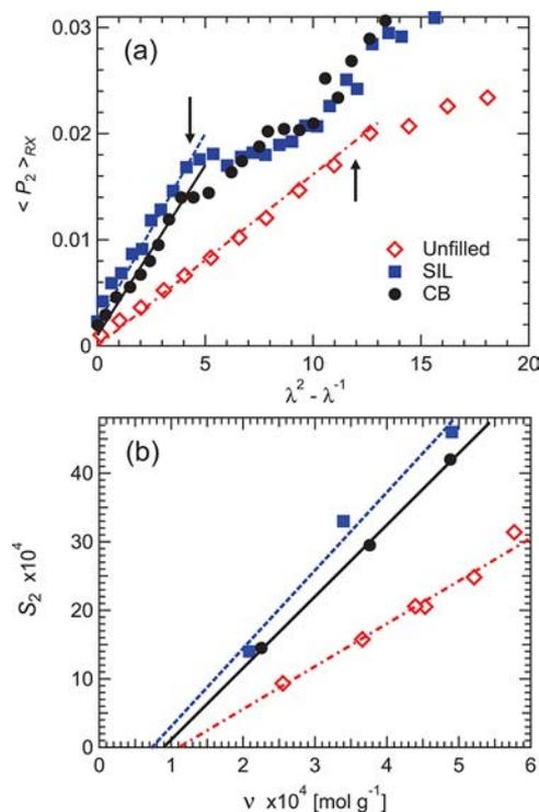
**Figure 4.** (a) Amorphous orientation parameter  $\langle P_2 \rangle_{RX}$  measured by X-ray scattering as a function of the elongation function  $\lambda^2 - \lambda^{-1}$  for systems with the same cross-link density: unfilled ( $\diamond$ ), SIL ( $\blacksquare$ ), and CB ( $\bullet$ ) samples. Crystallization onsets are indicated by arrows. (b) Slopes  $S_2$  of  $\langle P_2 \rangle_{RX}$  as a function of the cross-link density  $\nu$  measured by NMR.
