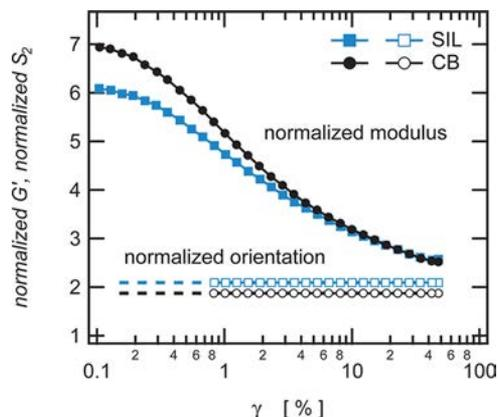
**Figure 5.** Storage shear moduli (full symbols) and slopes of the segmental orientation  $S_2$  (empty symbols) as a function of the tensile strain for two representative samples (■, SIL; ●, CB), normalized by the corresponding values in the unfilled sample with the same cross-link density. For the normalized moduli,  $\gamma$  is the amplitude of the oscillatory strain, for the normalized slopes,  $\gamma = \lambda - 1$ .
