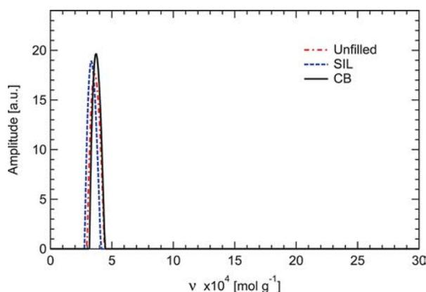
**Figure 7.** Distributions of cross-link density  $\nu$  in a pure, unfilled NR sample (1.0 phr S) and in SIL and CB filled materials (1.5 phr S), which have roughly the same average values  $\nu \approx 3.5 \times 10^{-4} \text{ mol}\cdot\text{g}^{-1}$ . No contribution from regions with cross-link densities up to 10 times the average value is observed.
