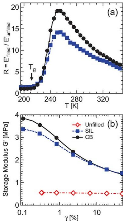
**Figure 1.** (a) Reinforcement in the linear regime at 10 Hz as a function of temperature and (b) oscillatory shear modulus  $G'$  as a function of the strain amplitude  $\gamma$  at 333 K and 10 Hz in unfiled ( $\diamond$ ), SIL ( $\blacksquare$ ), and CB ( $\bullet$ ) filled NR samples with 18.25% volume fraction of fillers. All samples have roughly the same cross-link density.
