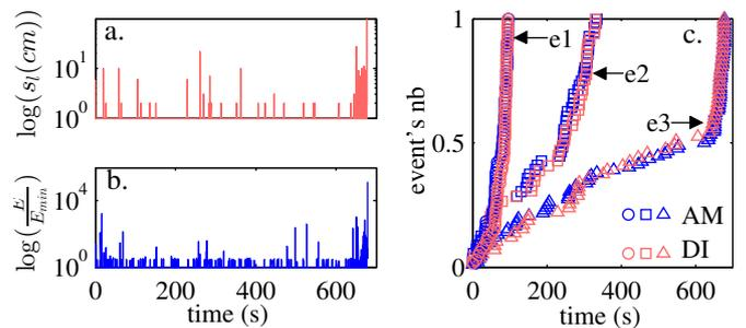
FIG. 2: Time series of (a)  $s_l$  and (b) the energy of AE during one experiment. (c) Comparison between DI activity and integrated AE activity for three experiments (e1, e2 and e3). The experiment represented in (a), (b) corresponds to experiment 3 in (c).
